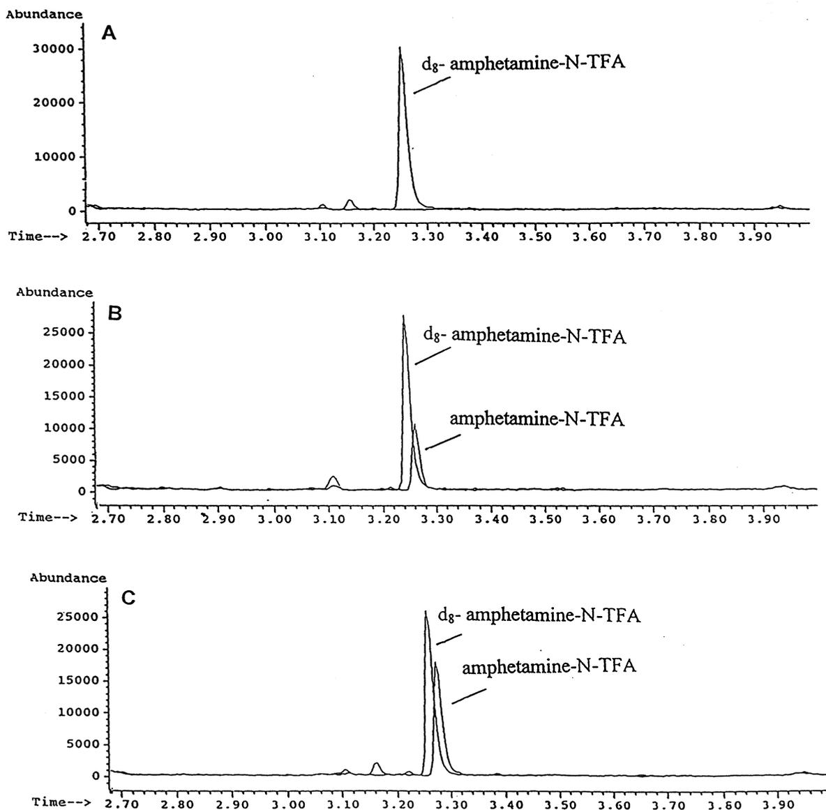
Fig. 2. Representative ion chromatograms for amphetamine ( $m/z$  118) and  $d_8$ -amphetamine ( $m/z$  143) of (A) plasma spiked (25 ng/ml) with  $d_8$ -amphetamine (ISTD), (B) Plasma spiked with amphetamine (10 ng/ml) and ISTD (25 ng/ml), and (C) plasma from a volunteer 1.5 h after oral administration of 20 mg of amphetamine (calculated concentration of 20.8 ng/ml) and ISTD (25 ng/ml).
